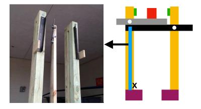
place by a piece of wood (blue). A rope attached approximately at the position shown with the arrow is pulled to activate the release. You may need a small block of wood or similar (X) at the bottom of the prop to prevent it from kicking back into the tower gap when the shot is triggered.
